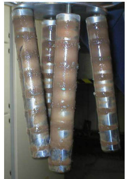
Magnets from a heavily contaminated oil circuit
