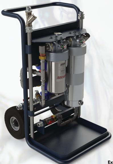
The FFC-3000 Fuel Filtration Cart is designed for dispensing, transfer and polishing filtration applications. Fully compatible with both diesel and bio-diesel, it combines a dirt tolerant progressive cavity pump with a large capacity particulate filter and high flow coalescing element to efficiently remove dirt and water from your fuel.
