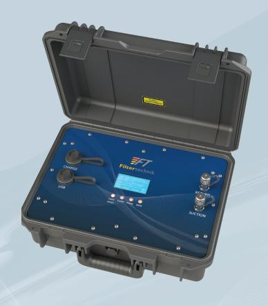
The FS9V2-PPM is fitted with an accurate laser counter for diesel fuels and moisture sensor to measure the PPM. The FS9V2-PPM-DEN model can measure PPM and density (kg/l) of any diesel fuel sample.
