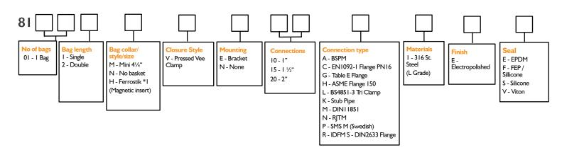
Example: 81011MVN10A1EE = 81 Series, Single Length Bag, MINI 41/2" Bag collar, pressed vee clampclosure, no mounting, 1" BSPM connections. 316LSt. Steel with electropolished finish and EPDM seals. Double length only.
