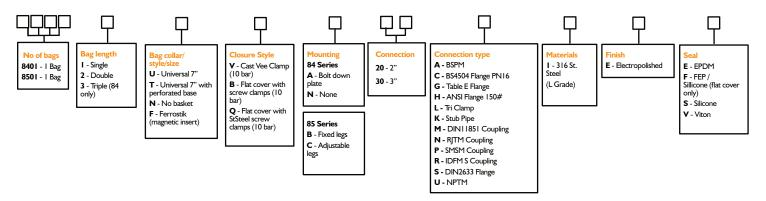
Example: 84011UVN20A1EE = 814Series, Single Length Bag, Universal 7" Bag collar, pressed vee clamp closure, no mounting, 2" BSPM connections. 316L St. Steel with electropolished finish and EPDM seals.
