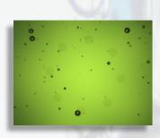
Air bubbles can be seen in images, which are size categorised and removed from particle counts.
