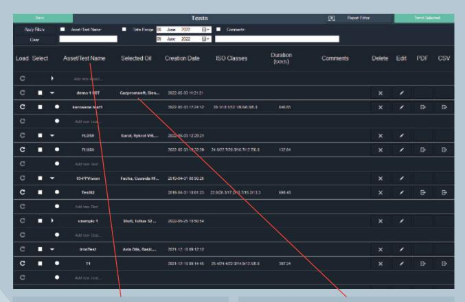
Create oil assets which then logs and records the data of completed tests. Refer back to this at any point as all the data is saved on the device. New tests are added and all data can be trended over time.
