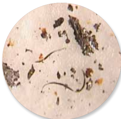
Particulate under microscope on a 1 micron patch
