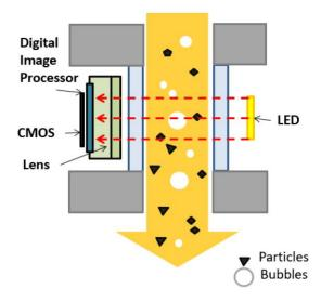
The sensor periodically captures images and processes these internally for the delivery of information to the user over Modbus.
