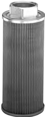
These all metal suction strainers are furnished with optimized pleat size and screen area for extended life and low pressure drop. 100 mesh stainless steel screen (140 micron) has 33.3% open area. Porting head is carbon steel, center core is plated perforated steel. End cap is heavy gauge zinc plated steel. These strainers can handle temperatures up to 250°F (121°C).
