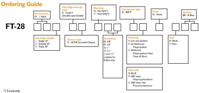
Example: 280100XN03BPNB = 28 Series, 1 x5" DOE cartridge, ACME screwed closure, No vent, 3/8"BSP'F' connections. All polypropylene construction with Nitrile gaskets.
