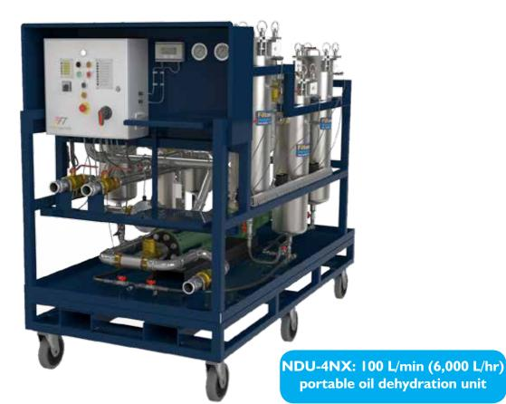
Our Neptune Dehydration Unit 4 is a transportable oil dehydration filtration unit capable of rapidly removing both free and entrained water to under 100ppm. The NDU-4NX is ideal for use around a plant & rugged enough to run continuously in order to clean up heavily contaminated oils.
